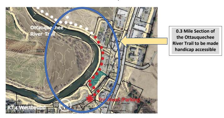
**Trailhead Ramp:** There is a 12" drop from the trailhead to the elevation of the initial 0.3 miles of the ORT. Currently there is a set of stairs to enable people to access ORT. These stairs do not accommodate wheelchairs or strollers. Because of this, we will need to construct an ADA-compliant ramp at the trailhead. The cost estimate for this ramp is \$10,000, which is approximately 80% for equipment rental and 20% for materials.
